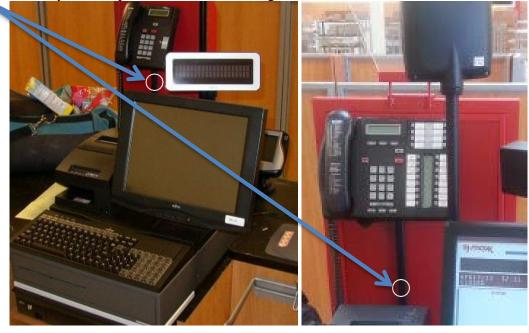
NOTE: The screws used to mount the phones MUST be ½ inch.
