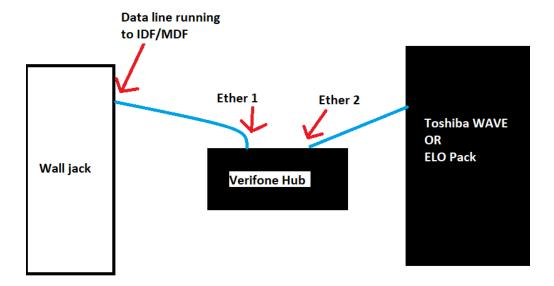
To connect the register and pinpad to separate ports:
