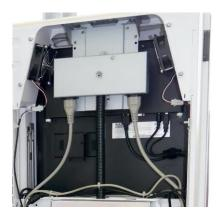
☐ Remove the top plate by unscrewing the four nuts.
