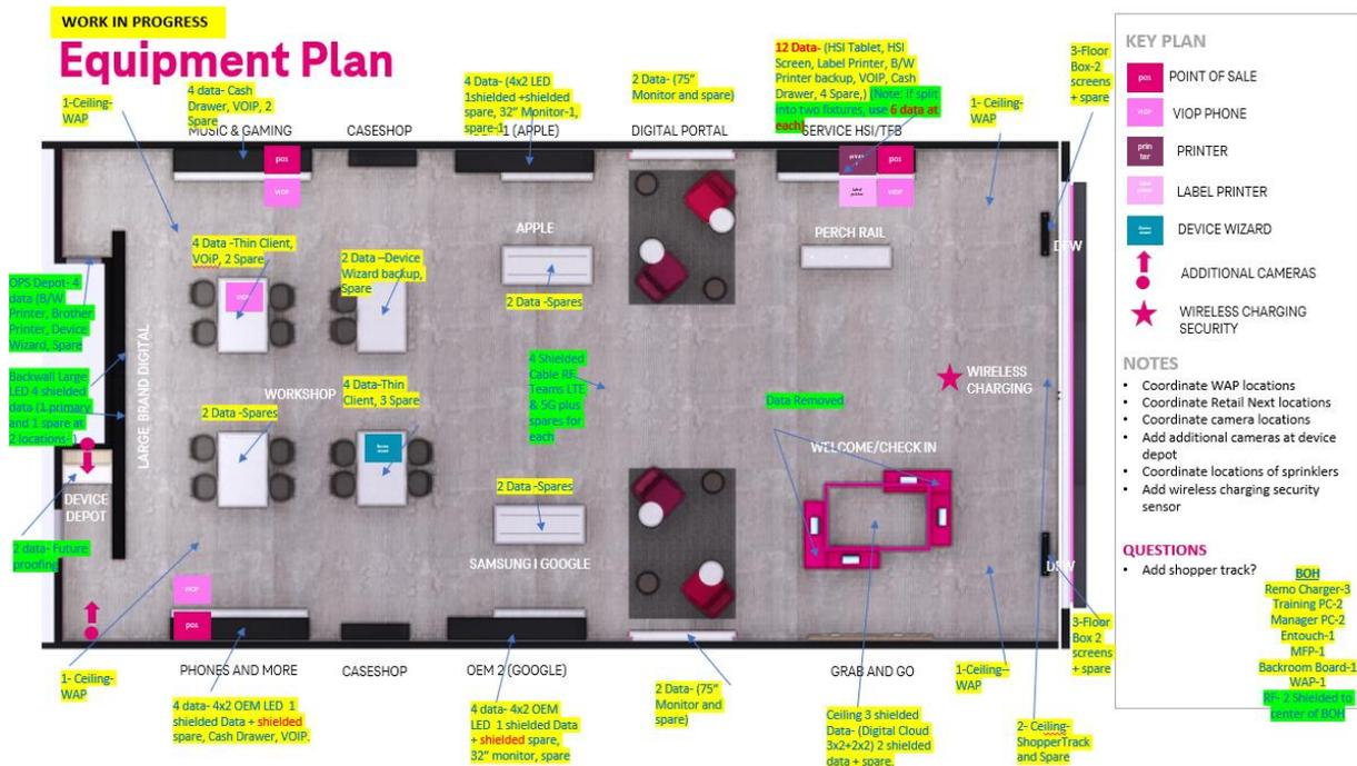
LV vendor is to coordinate rough-in timeline with construction GC but should be completed prior to the ceiling grid being installed on **Wednesday of week 3**. Field terminations must be completed prior to fixture delivery (**Monday of week 6**) to avoid access issues. All cabling is to be ran with **5'** service loops on both ends. RAN cabling to have 15ft service loops on both ends
