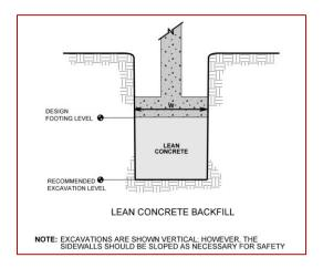
Over-excavation for structural fill placement below footings should be conducted as shown below. The over-excavation should be backfilled up to the footing base elevation, with engineered fill placed, as recommended in the **Earthwork** section.
